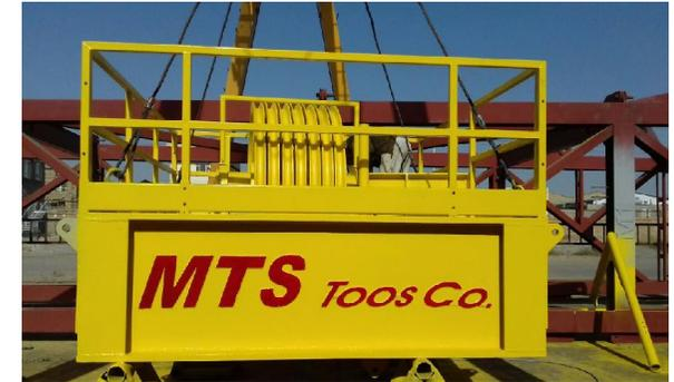
The **crown block** is the stationary section of a **block** and tackle that contains a set of pulleys or sheaves through which the drill line (wire rope) is threaded or reeved and is opposite and above the traveling block .
